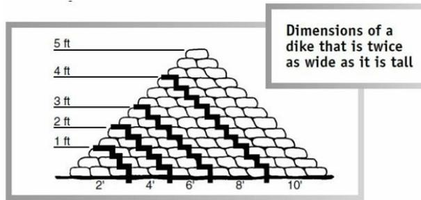
A common recommendation is to make the dike twice as wide as its height. This is a minimum width-to-height ratio that should be used. The estimated number of bags needed for this ratio is in the following table. This is based on each bag having placed dimensions of about 4 to 5 inches high by 9 to 10 inches wide by 14 inches long.
