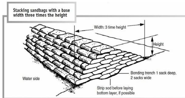
Use the following equation to estimate the number of bags required per linear foot of dike for a dike with a **base width that is three times the height**.
